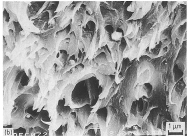
Figure 8 (a–c) Scanning electron micrographs taken from various locations of the fracture surface obtained in a statically loaded specimen carried out at -196^{\circ}\text{C} .
