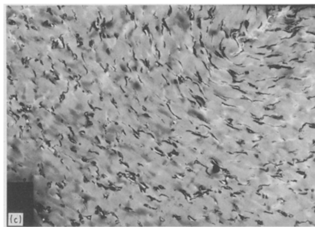
Figure 12 (a–c) Transmission electron micrographs taken from an ultra-thin section of an impact-loaded specimen at 70°C. Fracture behaviour is seen to be cavitation and shear yielding. No crazing is found. Crack tip is at the top right-hand corner of (c). Details are given in the text. (a) \times 13\,600 , (b) \times 10\,300 , (c) \times 3000 . 12(c).
